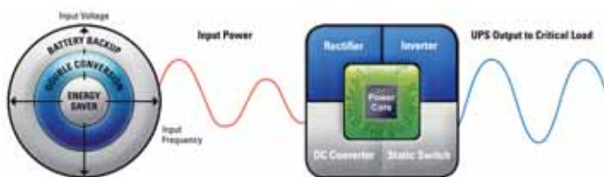
Input power quality within rectifier tolerance
