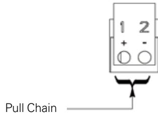
**Figure 4-13. Pull Chain Terminal Block Connector Assignments**
