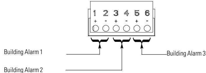
Figure 4-11. Building Alarm Terminal Block Connector Assignments
