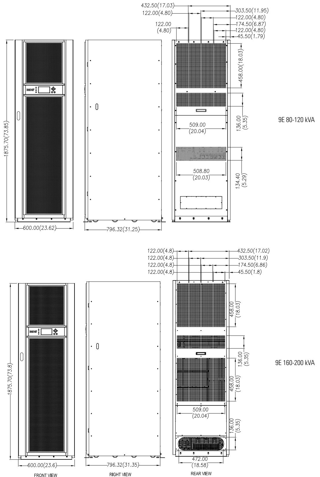
**Figure 3-1. UPS Cabinet Dimensions (Front and Right Side Views)**
