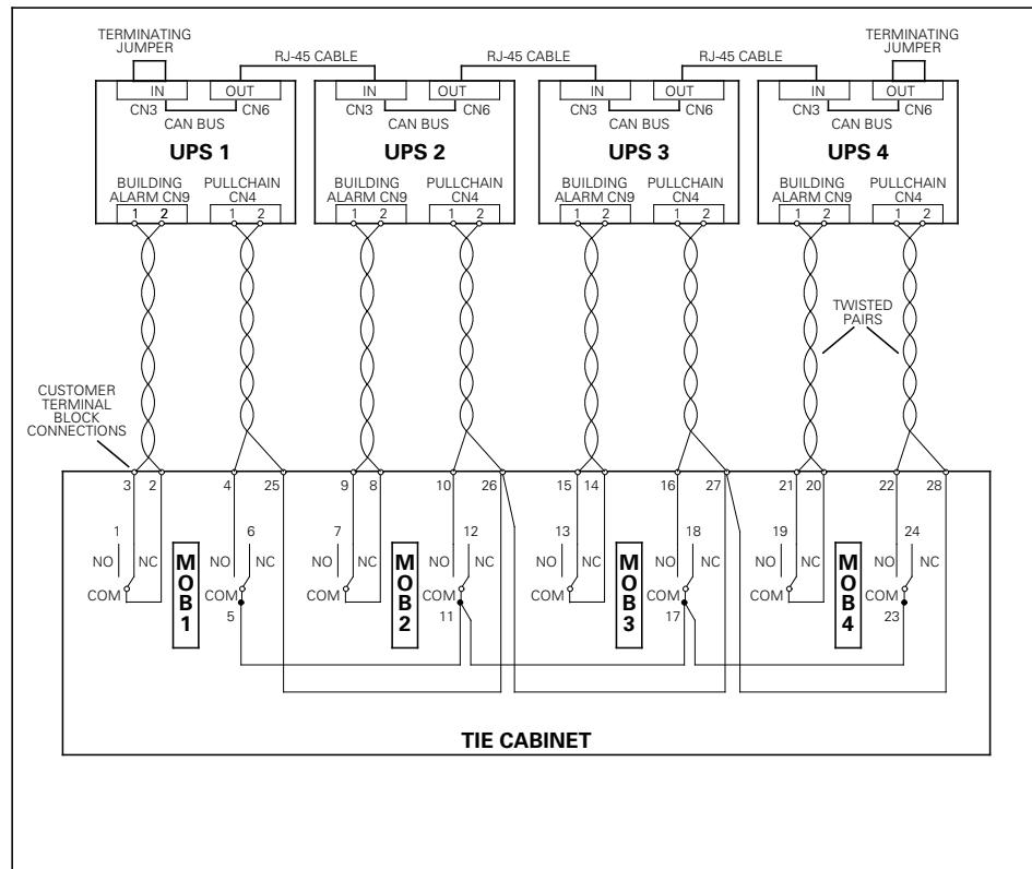
Figure 4-14. Parallel UPS Control Wiring
