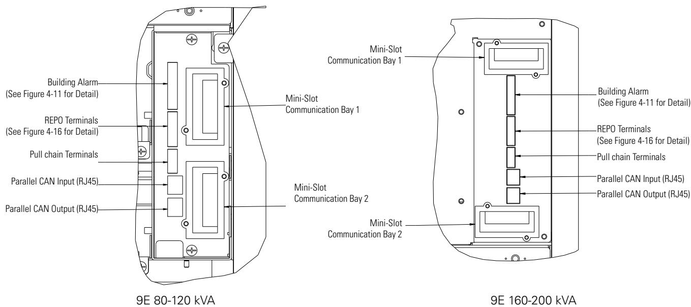
Figure 4-10. Interface Terminal Detail (Terminal Cover Removed)
