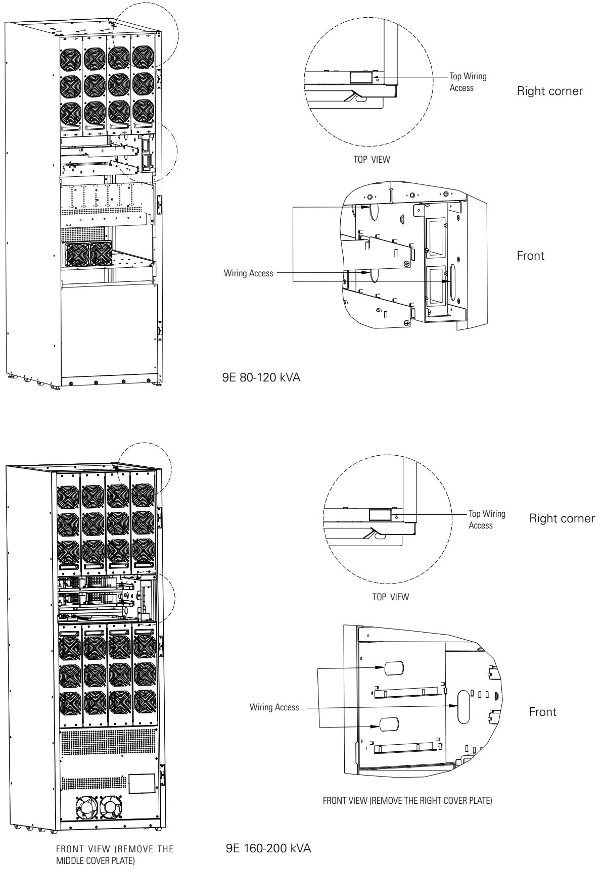
**Figure 4-12. Interface Wiring Access**
