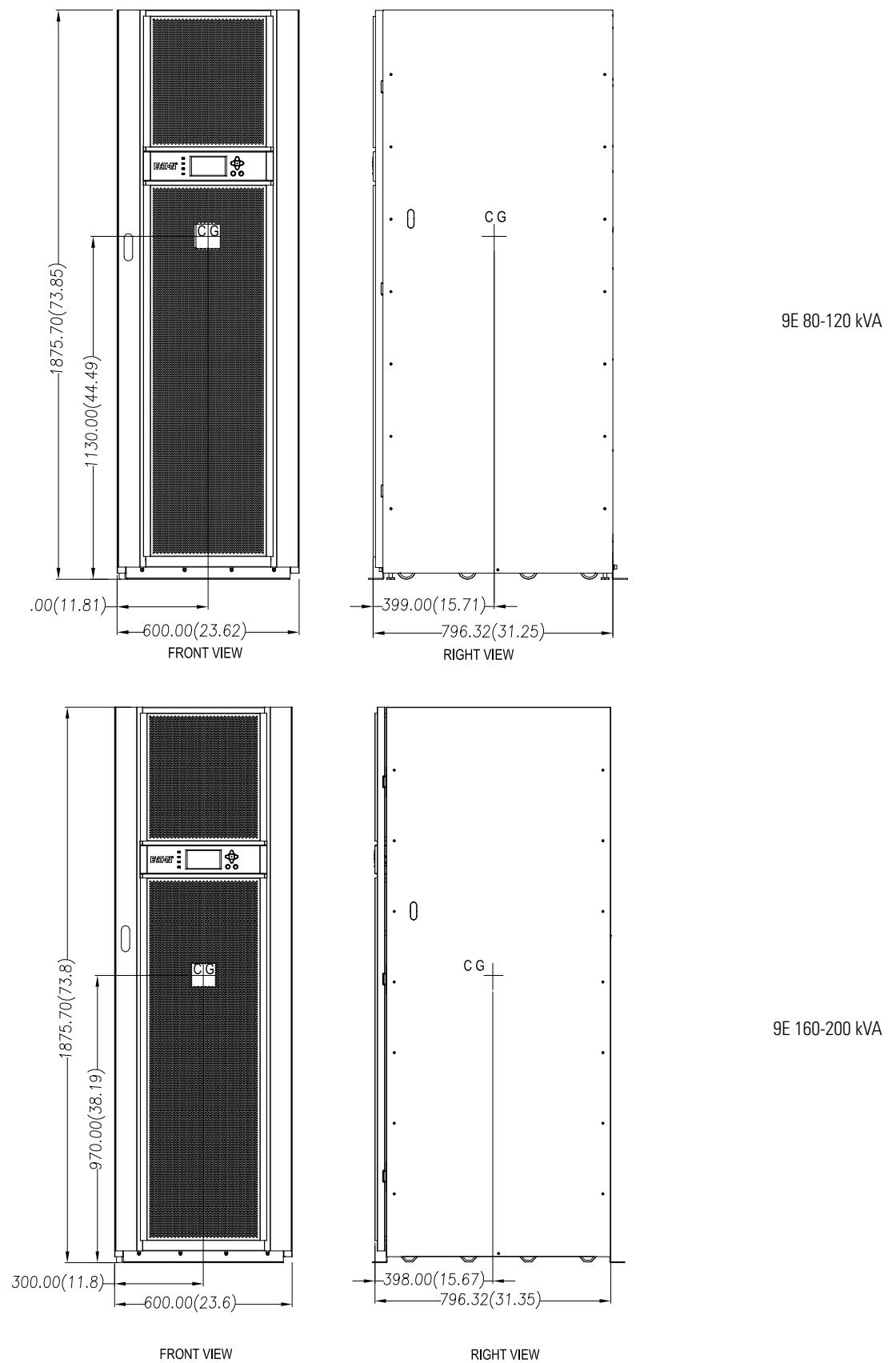
**Figure 3-3. UPS Cabinet Centre of Gravity**
