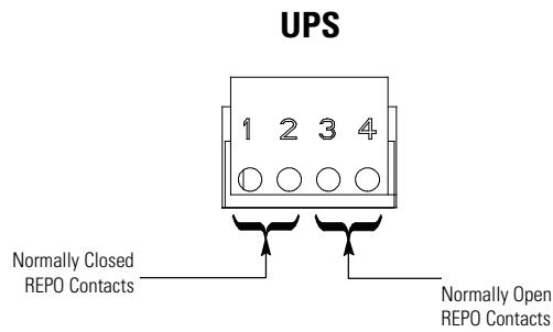
**Figure 4-16. REPO Terminal Block Connector Assignments**
