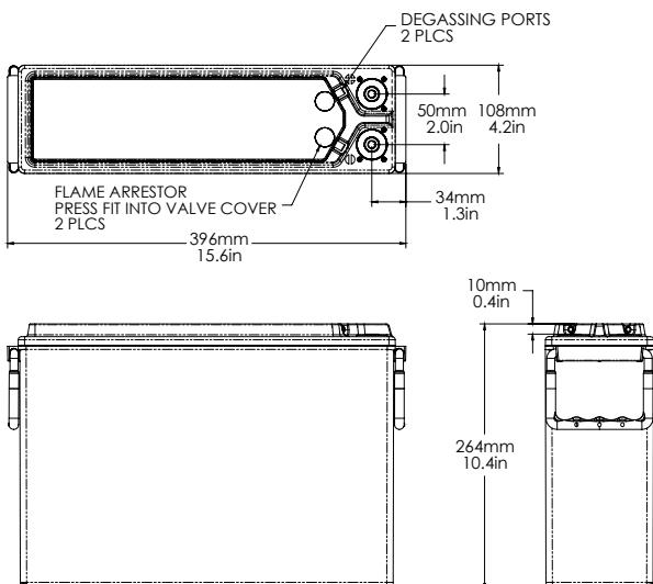
All NorthStar batteries are compliant with: Telcordia SR4228, IEC 60896; Bellcore GR-63-Core, Issue 1; British, German, and Russian telecom standards; UL approved. NorthStar is registered to ISO 9001 and ISO 14001.
